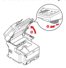
**4.** Press the cover release (a) and open the top cover (b) fully.
